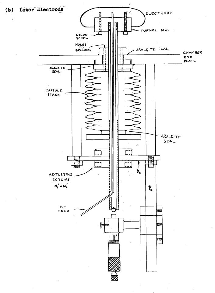
the two pairs of large bevelled nuts  $(N_1 \ N_2 \ and \ N_1' \ N_2')$  on the electrode shafts against fixed mild steel discs  $(D_1 \ and \ D_2)$  causing the bellews to be expanded or contracted and hence the electrode spacing to be varied.
