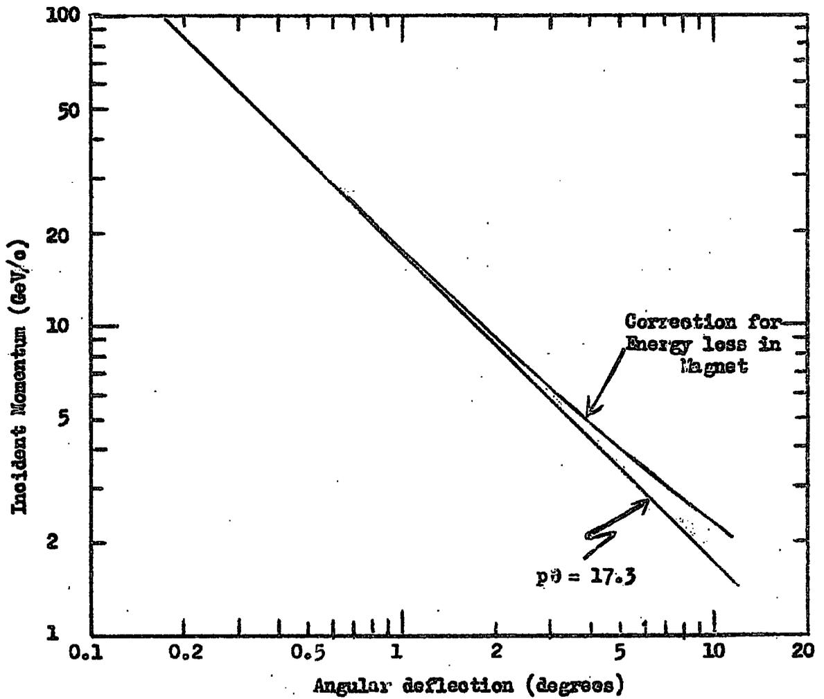
Fig. 3.2 The relationship between the incident momentum and angular deflection for the present experimental arrangement.
