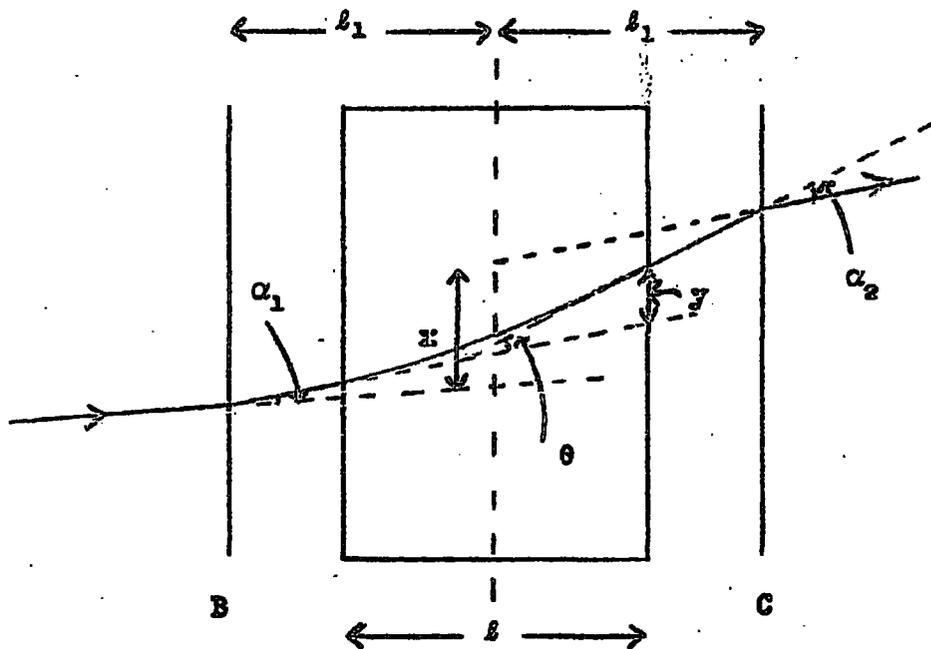
Fig. 3.6 Scattering of a particle in the magnet and flash-cube trays.
