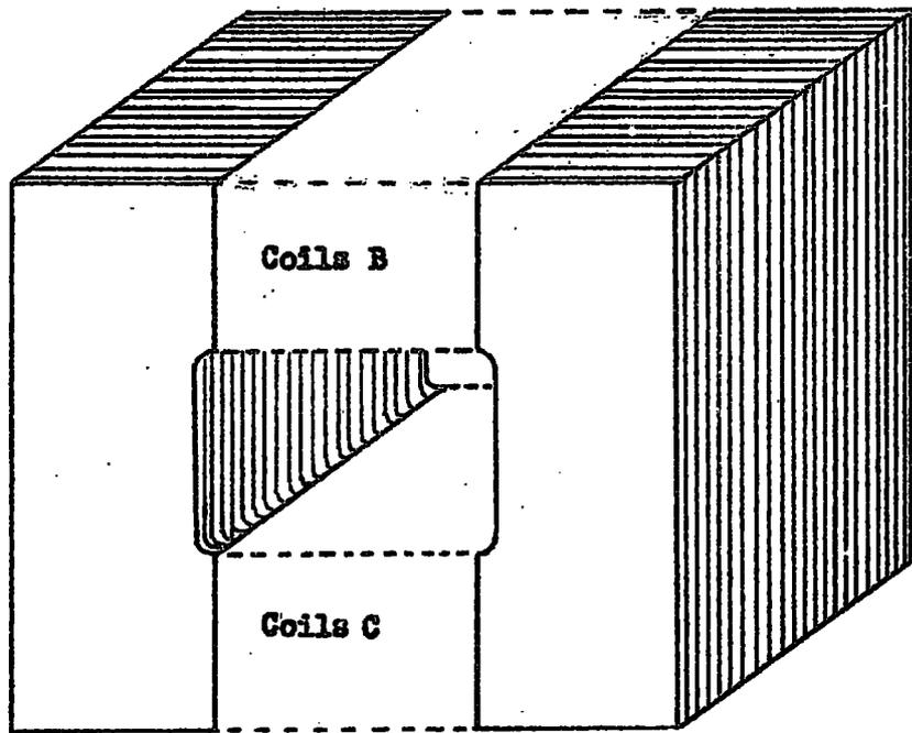
Fig. 2.1 The solid iron magnet.
