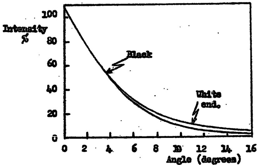
Fig. 2.9 (b) Polar diagram for light output from the flash-tubes.
