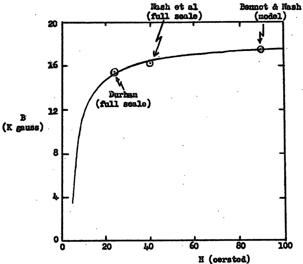
**Fig. 2.6 Comparison of the operating values for the various solid iron magnets.**
