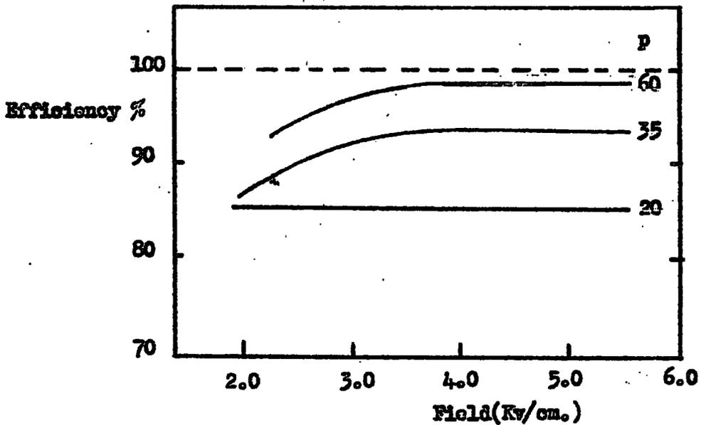
Fig. 2.7(a) The efficiency, field characteristics, with gas pressure (cm.Hg) as parameter.  $T_D = 3.2 \mu\text{sec}$ ;  $T_R = 0.5 \mu\text{sec}$ ,  $\tau = 4 \mu\text{sec}$ .
