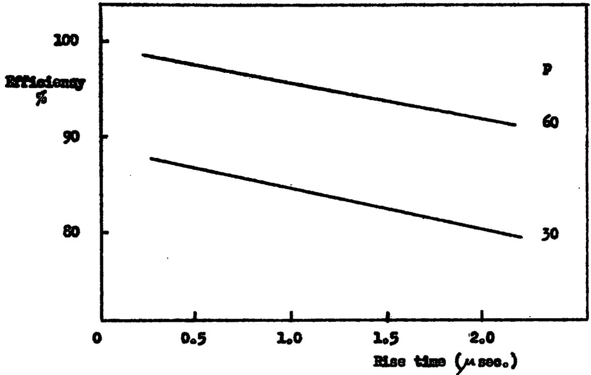
Fig. 2.8 (a) The efficiency, rise time characteristic, with gas pressure ( cm.Hg ) as parameter.  $E_{max} = 3.0 \text{ Kv/cm}$ ,  $T_D = 3.2 \mu\text{sec}$ ,  $\tau = 4 \mu\text{sec}$ .
