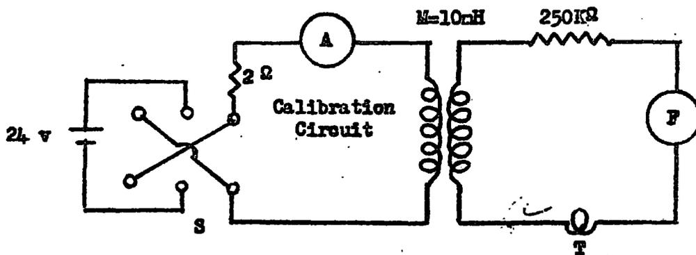
Fig. 2.4 Circuit used to calibrate the fluxmeter F and measure the magnetic induction. (S is the reversing switch).
