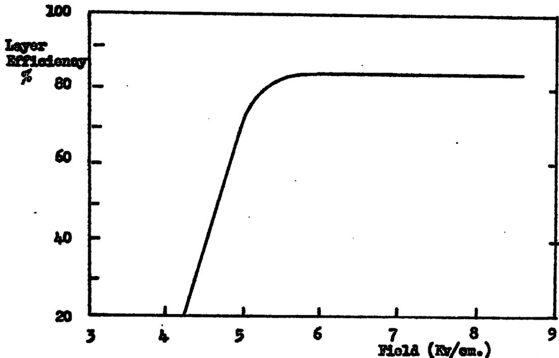
Fig 2.8 (b) The layer efficiency, field characteristics for the tubes used in the horizontal spectrograph.
