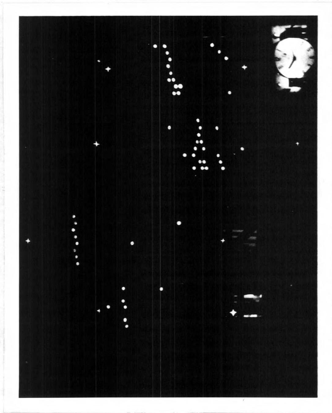
Plate 6 The track of a 1180 GeV/c (approx) positive muon incident at  $87.5^\circ$  to the zenith, with a knock-on electron in tray A.
