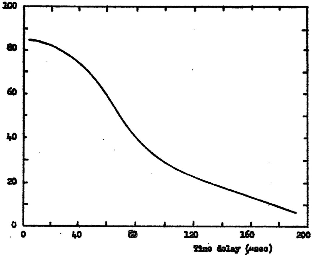
Fig.2.9 (a) The efficiency, time delay characteristic for the tubes used in the horizontal spectrograph.
