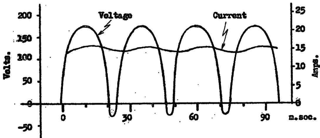
**Fig.2.3** Characteristics of the current and voltage supplies to the magnet windings.
