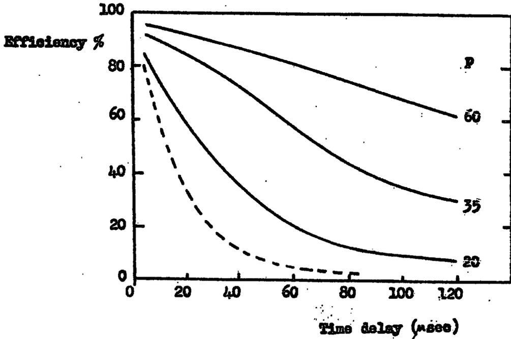
Fig. 2.7(b) The efficiency, time delay characteristics, with gas pressure (cm.Hg) as parameter.  $E_{\text{max}} = 3.7 \text{ Kv/cm}$ ,  $T_R = 0.5 \mu\text{sec}$ ,  $\tau = 4 \mu\text{sec}$ .
