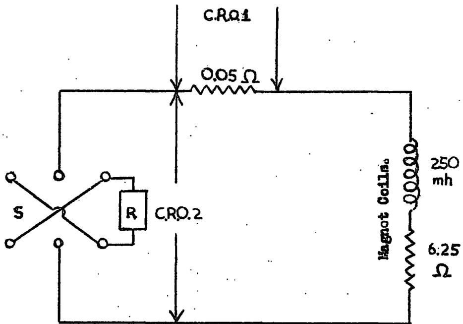
**Fig.2.2** Circuit used to examine the characteristics of the power supply to the magnet coils. (R is the rectifier, and S the reversing switch.)
