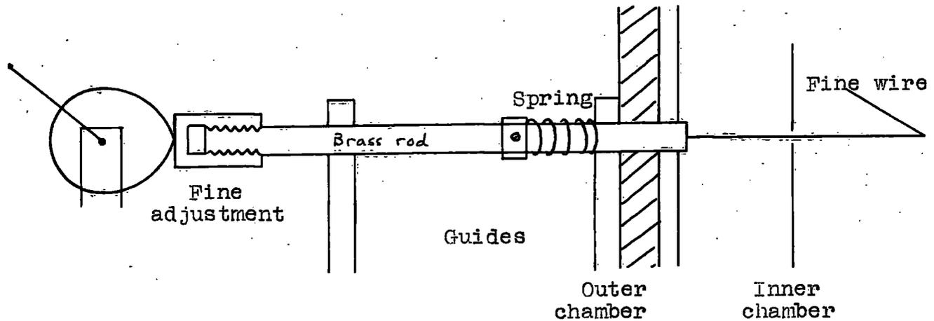
Fig. 7 Contact Mechanism
