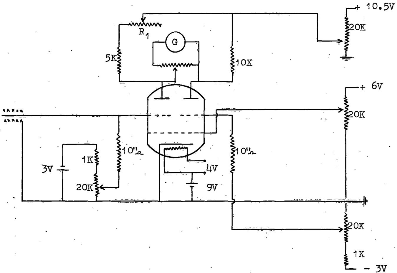
Fig. 8 Balanced Electrometer Tube Circuit
