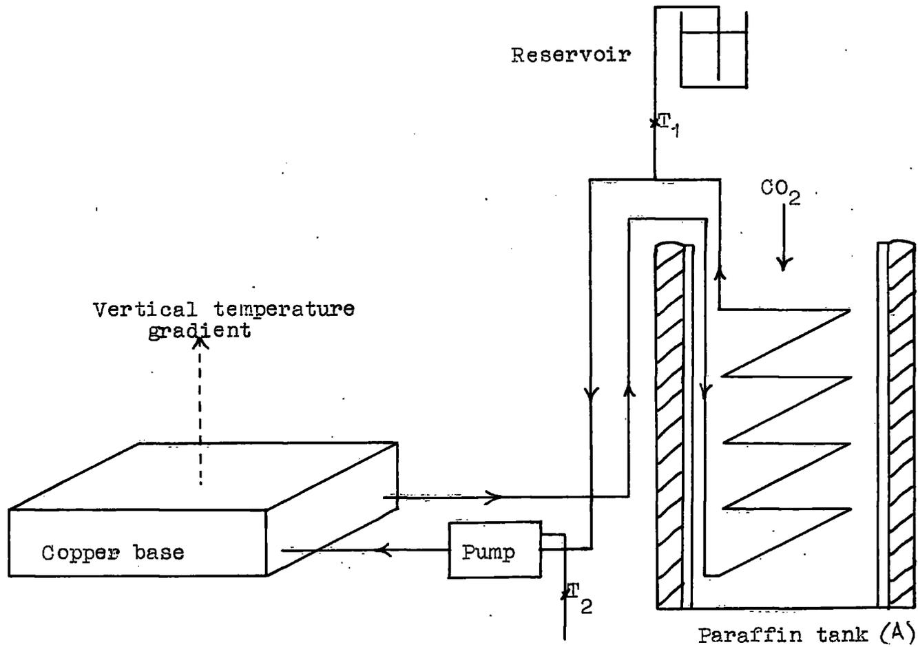
Fig. 1 The Cooling System
