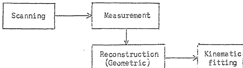
Initially the photograph taken is projected onto a screen and the image scanned for events and tracks leading from these events.
