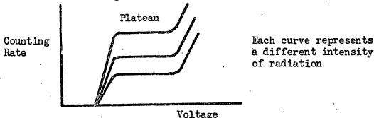
Fig. 2.3 Geiger Counter: Counting Rate Versus Applied Voltage
